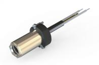
FEINMETALL high-voltage contacts were developed for contacting e-mobility plugs and sockets in the automotive sector. The probes are used for contacting pin, socket & shield contacts under high voltage conditions up to 5000V DC and combine several test possibilities in one probe.
