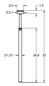
The receptacle H100 can be used for mounting.
